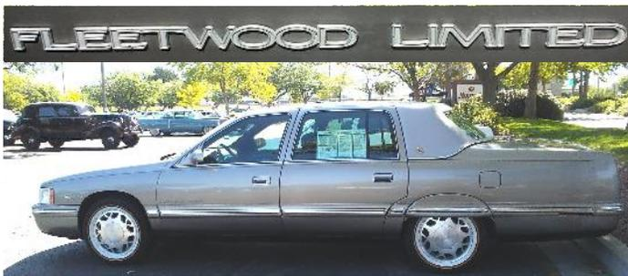
The labor-intensive effort was performed by Superior Coach Company of Lima, OH. They specialized in Cadillac alterations and are better known for their limos and funeral cars. Modifications include, but are not limited to, cutting and extending the wheelbase by three inches and the roof by six inches. This enables a roomier rear compartment, providing for an inlaid wooden writing table on the passenger-side and
