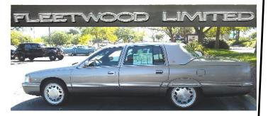
The labor-intensive effort was performed by Superior Coach Company of Lima, OH. They specialized in Cadillac alterations and are better known for their limos and funeral cars. Modifications include, but are not limited to, cutting and extending the wheelbase by three inches and the roof by six inches. This enables a roomier rear compartment, providing for an inlaid wooden writing table on the passenger-side and
