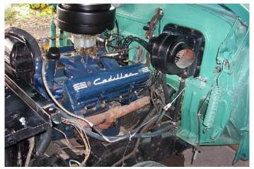
I had the distributor on the work bench and was examining it for the umpteenth time, when I finally noticed the tang on the distributor shaft that mates with the cam gear was off center by a nearly imperceptible amount to prevent being installed the way I had installed it. I had had to use more force than I should have to seat it. I removed the intake manifold and valley cover and rotated the gear 180 degrees. Once that was accomplished the wobble was gone.
