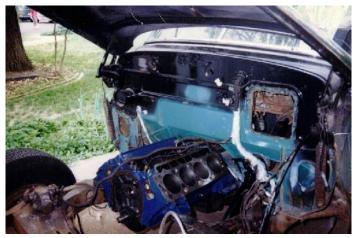
When the engine was reassembled, I tried for a long time to start the car without success, and after much investigation, I concluded that the engine was 180 degrees off in the timing. When reassembling the engine, I had assumed the timing marks lined up when the #1 cylinder was at top dead center ready to fire. I finally found a sentence in the repair manual (not where I would have expected to find it) that said the timing
