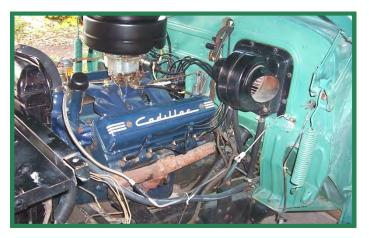
I had the distributor on the work bench and was examining it for the umpteenth time, when I finally noticed the tang on the distributor shaft that mates with the cam gear was off center by a nearly imperceptible amount to prevent being installed the way I had installed it. I had had to use more force than I should have to seat it. I removed the intake manifold and valley cover and rotated the gear 180 degrees. Once that was accomplished the wobble was gone.
